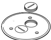
**Brass Cover Plate – With two screw plug openings, 5 1/2" [140mm] diameter for carpet.** Screw plug openings are 1 1/2" [38mm] – 16 tapped openings.
