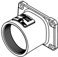
**2" Conduit Transition Hub** – Trade size 2" die cast zinc conduit fitting allows for 2" conduit to transition into a shallow box design. Includes: die cast fitting gasket. Accepts standard 2" threaded conduit or trade size EMT and PVC conduit fittings.
