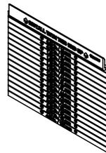
**Divider** – Used to isolate power and low voltage (communications and audio/video) compartments. Graduated markings indicating location to cut divider to, in order to match concrete pour.
