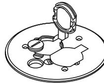
**Dual-Service Brass Duplex Cover Plate** – With flip lids. Supplied with 1/2" [12.7mm] screw plug for accessing communication cables. 5 1/2" [140mm] diameter for **carpet applications only**. Used in conjunction with the 881DIV to complete dual-service activation.
