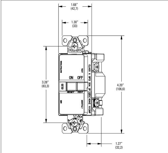
Figure 9. SGFD20 Line art with dimensions
