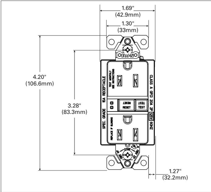
Figure 1. SGF15, SGF15-M & SGF15F Line art with dimensions
