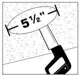
**Step 1:**Using provided stencil, trace cutout lines for housing hole on ceiling. Use saw to make appropriate 5-12" cutout.
