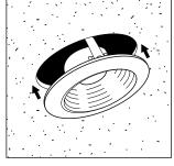
**Step 4:** Insert trim into housing, and screw in lamp.
