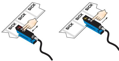
Press both the "+" and "-" buttons together, hold > 1 s and then release the teach-in buttons. The red LED flashes.
