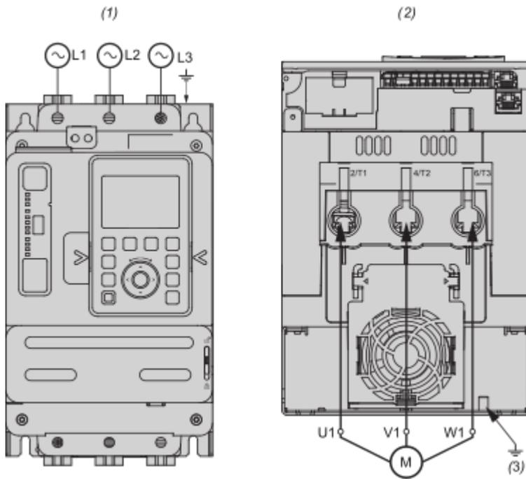
Use class C cables for the power connections.
