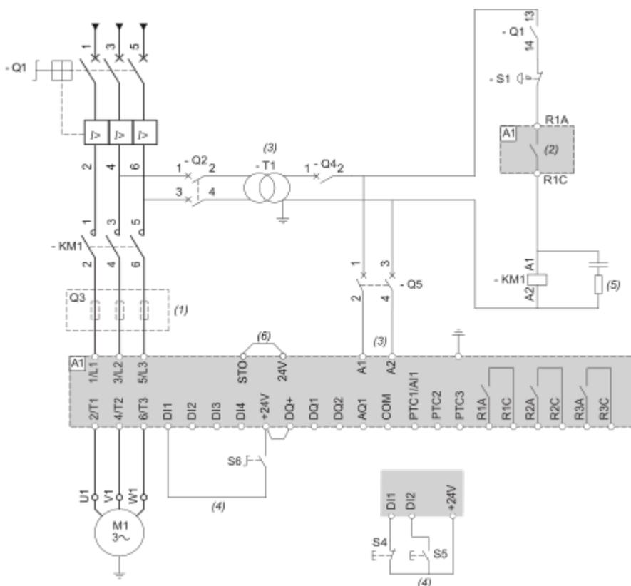
(1) : Installation of additional fast-acting fuses is mandatory to upgrade to type 2 coordination according to IEC 60947-4-2.
