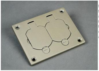
Nickel powdercoat duplex cover plate, for OmniBox® and Modulink™ Series floor boxes. Cover plate is 3.290 inch x 4.310 inch (83.6mm x 109.5mm). Flip lids can also be used with 106 type frames for communications. NOTE: Brass covers and flanges are not interchangeable with aluminum or nonmetallic covers and flanges. Nonmetallic covers are interchangeable with aluminum flanges. Made in USA.
