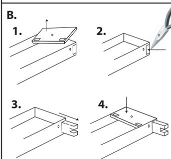
**B) Side Socket Mount** - Remove the metal end top plate as mentioned in style A. Remove the knockout tab on the side of the housing. Push the socket so that it snaps into the new slot on the side of the housing. Re-attach the metal end top plate to the housing.
