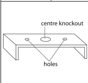
3. Turn the fixture over and locate the center knockout. Make sure the fixture is supported on the underside and break part of the knockout away using a hammer and screw driver. Twist out the knockout using pliers.
