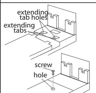
**Note:** Toggle bolts will require a larger pilot hole. Secure the fixture to the ceiling using the appropriate fasteners. Connect the ground wire to the ground screw located near the center knockout. Connect the black wire from the fixture to the black wire from the electrical box. Connect the white wire from the fixture to the white wire from the electrical box. Once wires are connected, carefully tuck wires and marretts into the metal outlet box.
