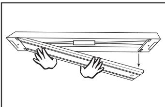
1. Remove the wire cover by loosening the screw.
