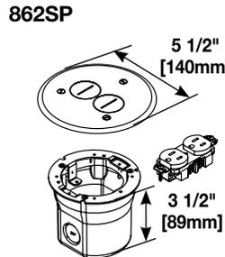
**PVC Floor Box Assembly for Wood or Concrete Floors** – Includes 862 Series Floor Box, one 15A, 125V tamper-resistant brown duplex receptacle, and one 895SP brass cover for carpet. Cover provides two 1 1/2" [38mm] screw plug openings.
