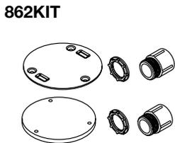
**Concrete Floor Kit** – When using any of the 862 Series Floor Boxes in a concrete floor, the 862KIT will provide a mud cap for the concrete pour, two 3/4" trade size conduit hubs, and a scrub water gasket.
