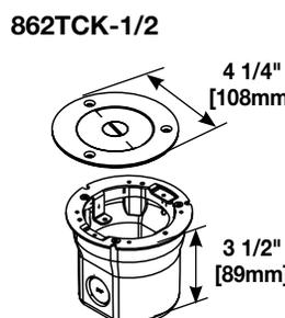
**PVC Floor Box Assembly for Wood or Concrete Floors** – Includes 862 Series Floor Box and one 896TCK-1/2 brass cover for tile. Cover provides one 2 5/8" [67mm] and one 1/2" [12.7mm] concentric screw plug openings.
