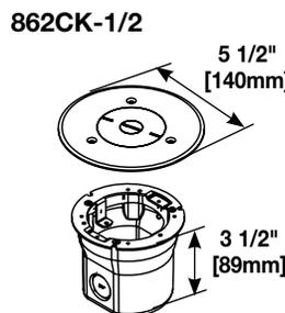
**PVC Floor Box Assembly for Wood or Concrete Floors** – Includes 862 Series Floor Box and one 896CK-1/2 brass cover for carpet. Cover provides one 2 5/8" [67mm] and one 1/2" [12.7mm] concentric screw plug openings.
