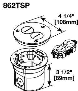
**PVC Floor Box Assembly for Wood or Concrete Floors** – Includes 862 Series Floor Box, one 15A, 125V tamper-resistant brown duplex receptacle, and one 895TSP brass cover for tile. Cover provides two 1 1/2" [38mm] screw plug openings.
