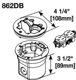
**PVC Floor Box Assembly for Wood or Concrete Floors** – Includes 862 Series Floor Box, one 15A, 125V tamper-resistant brown duplex receptacle, and one 895T brass duplex receptacle cover for tile.
