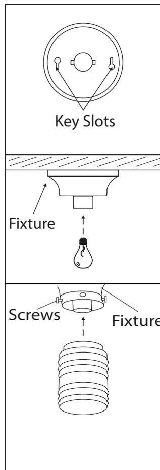
3. Tuck the electrical wires into the electrical box and position the "key slots" over the support screws. Turn and lock the support screws into the "key slots". Tighten the support screws into place.
