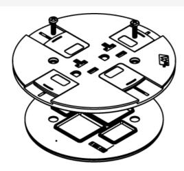
Nonmetallic slide holder assembly. Available in black (BK), gray (GY), ivory (VY), nonmetallic brass (BS), and nonmetallic aluminum (AA). Assembled with scrub water gasket. For use on tileor carpet floors.
