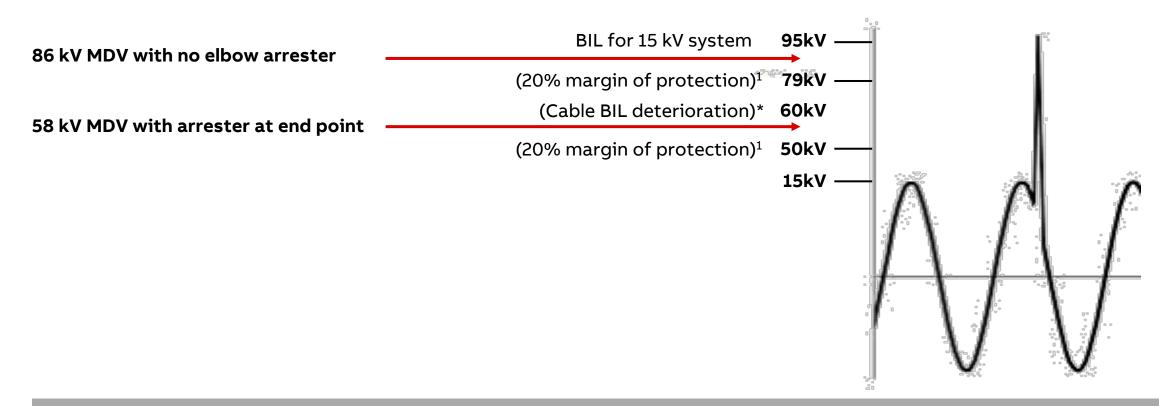
To reduce the total surge voltage to a value below 50 kV, additional arresters are required in the system.
