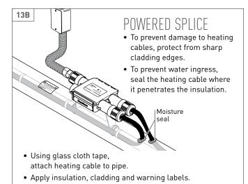
• Terminate power wiring in user-supplied junction box.
