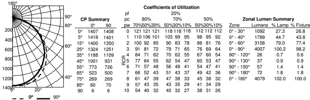
EPANL 22 34L 40K, 3479 delivered lumens, tested in accordance to IESNA LM-79.
