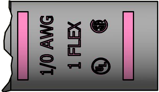
DETAIL E BOTTOM INK MARKING
