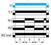
Function Di: Symmetrical Flasher Relay (Starting Pulse On)
