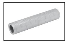
HYSPLICE™ sleeve designed to withstand jumper loop tensile and vibration stresses up to 60% RBS. Made of aluminum with staked-in cable stop. Installed with same die as equivalent full-tension sleeve. Made from electrolytic grade aluminum. Surface oxides removed at factory and sealed.
