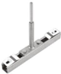
This system is designed to reduce cable pulling by allowing access from both sides of cable tray. Installation cost and time are reduced significantly by single-point suspension.
