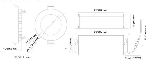
Hole cut size Ø3 <sup>5</sup>/<sub>8</sub>" (90mm)
