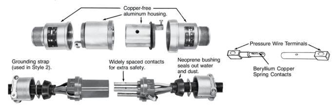
**Energized contacts** deeply recessed to reduce danger of accidental touching, minimize possibility of exposed arcs. Insulator quenches arcing, and is resistant to abnormal heat and to fire.
