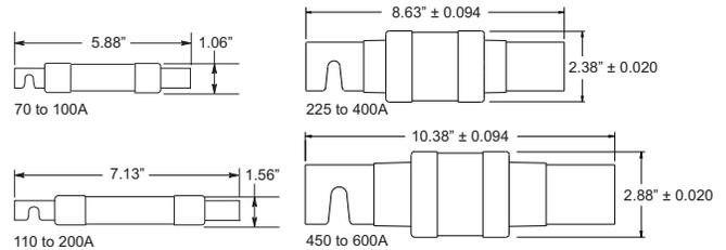
**Description:** Advanced protection, energy efficient Class RK5 dual element, current-limiting, time-delay fuses. Time-delay – 10 seconds (minimum) at 500% of rated current.
