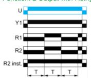
Function Di: Symmetrical Flasher Relay (Starting Pulse On)
