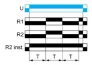
Function: 1 Output with Retrigger / Restart Control
